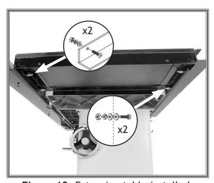
Figure 19. Extension table installed.
